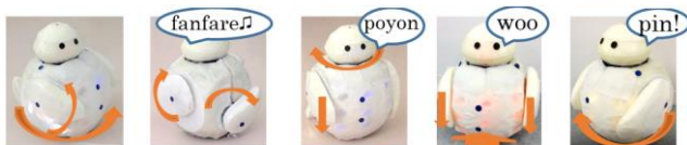
(a)behavior + color (b)behavior + sound (c) emotion Fig. 4 Example of the robot's behavior
